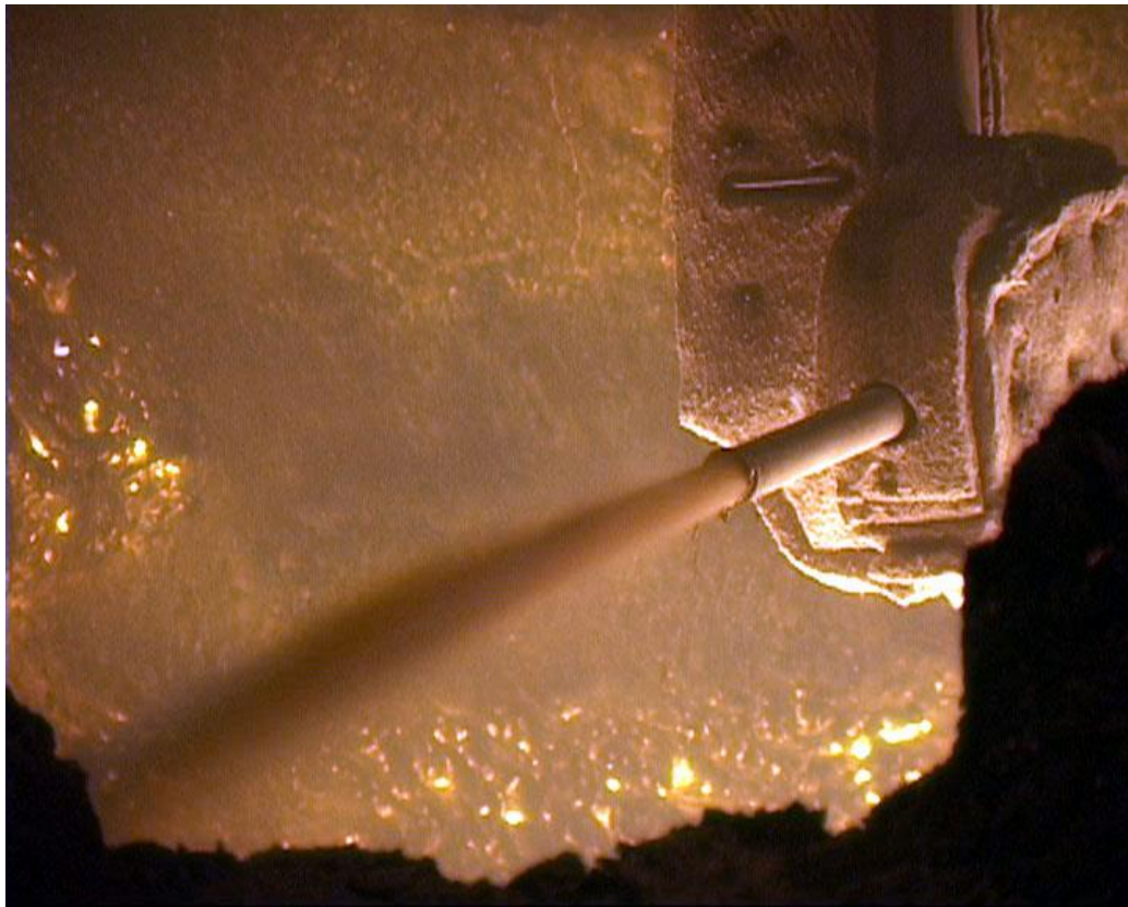
Figure 2: Application of magnesia “gunning mix” (source: www.grecianmagnesite.com/.../files ).
