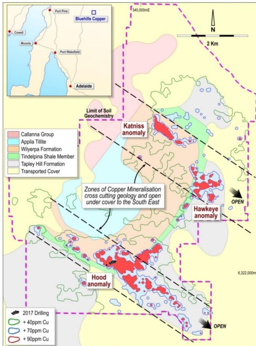
Figure 1: Blue Hills location map showing copper mineralisation and areal extent of Blue Hills magnetic anomaly.
