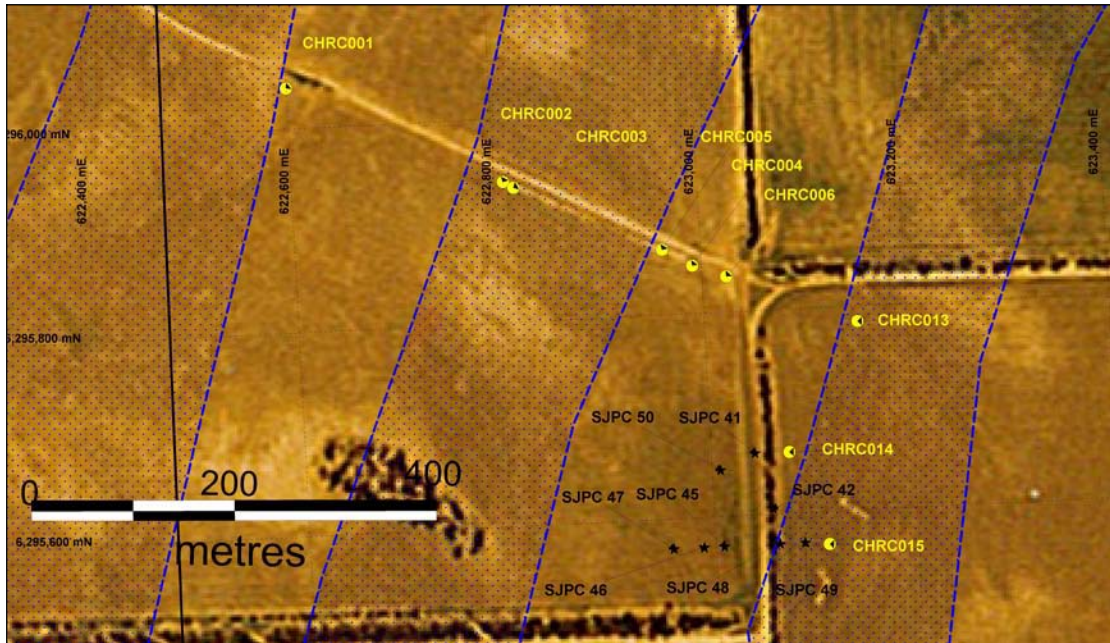
Figure 1: Location of RC drill holes drilled at Jamieson Tank. Yellow indicators are holes drilled by Archer, black indicators are historical drill holes drilled by WMC. Blue shaded areas represent the high magnetic units
