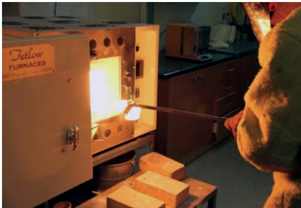
Removing Archer’s dead burned magnesite from furnace.
