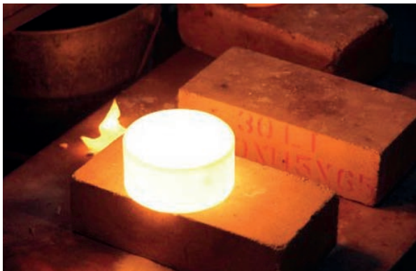
Cooling of Archer’s dead burned sample.
